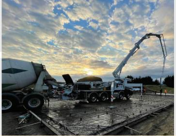
Machines from this class utilise their full potential on the construction site: flexible booms with 4 or 5 arms that can operate precisely inside low buildings, tunnels or under bridges, with an unfolding height of below 4 m. Ideal for extremely efficient operation on small and medium construction sites.
